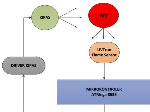
Gambar 6. Diagram Blok Skema Sistem Pendeteksian Api
