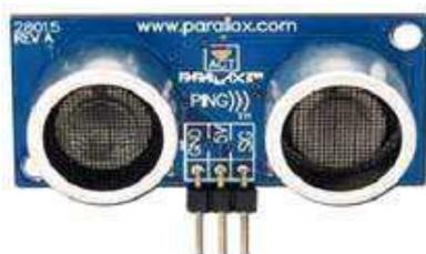
Gambar 2. Sensor Jarak Ping Ultrasonic
