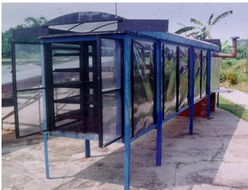
Gambar 4. Pengering lorong hibrid energi surya-biomassa terpadu
