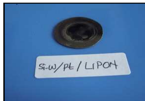
Figure 10. A thin layer of electrolyte LiPON on Pt on Si-wafer substrates obtained by by RF Sputtering. also looks uneven, but it is being optimized to obtain a more homogeneous layer
