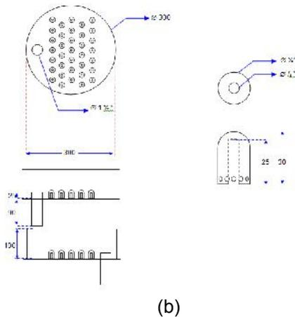
**Gambar 10** – Kolom Destilasi (a) Kolom Beer (b) Kolom Rectifier
