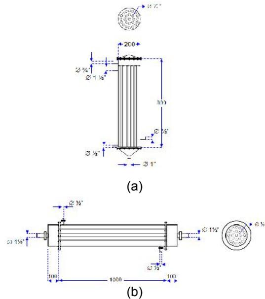
**Gambar 11** – (a) Pre Heater (b) Kondensor
