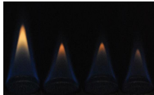
Equivalence ratio ( \phi ) pola api bunsen burner
