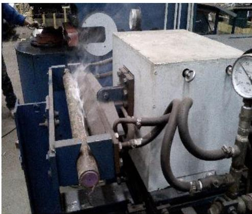
Gambar 2. Mesin Induction Heating
