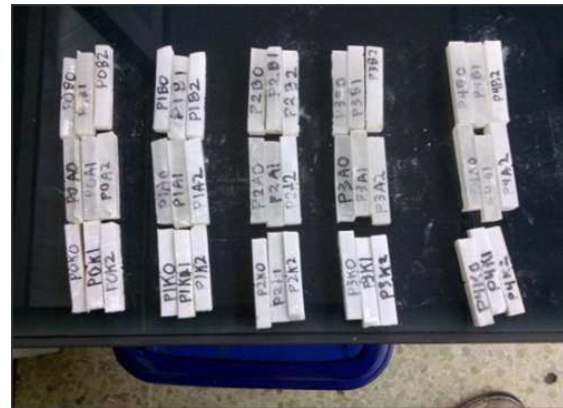
Gambar 2: Sampel uji charpy
