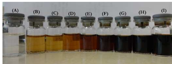
Figure 2. Solution of carbon nanoparticles for various concentration, (A) 0 g; (B) 0.005 g; (C) 0.001 g; (D) 0.025 g; (E) 0.05 g; (F) 0.1 g; (G) 0.2 g; (H) 0.3 g; (I) 0.4 g, at 20 ml of sea water
