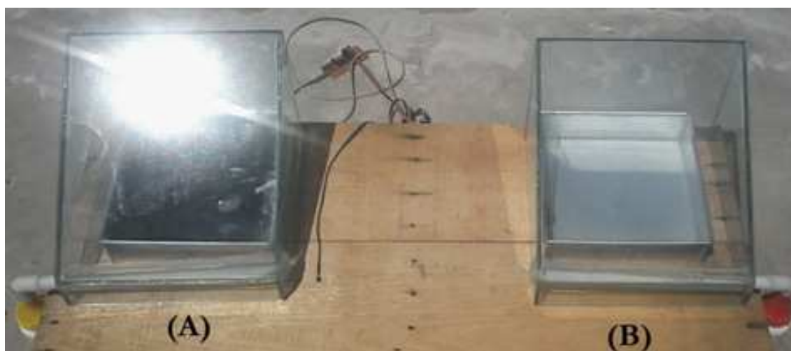
Figure 5. Solar distillation reactor (A) with the carbon nanoparticle, (B) without carbon nanoparticle addition.
