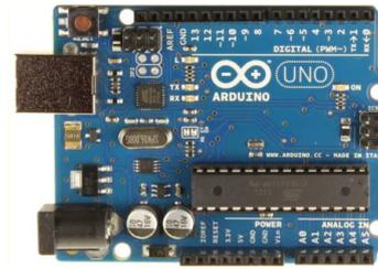
Gambar 4. Board Arduino UNO
