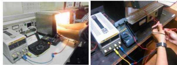
Gambar 19. Proses Pengukuran Suhu Resistansi Resistor
