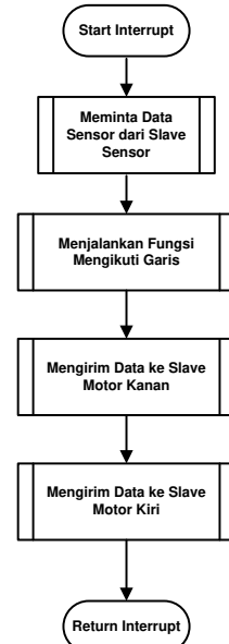
Gambar 12. Flowchart Program Mikrokontroler Master
