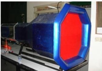
Gambar 3.2 Settling Chamber
