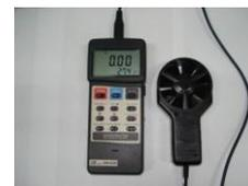
Gambar 3.5 Anemometer
