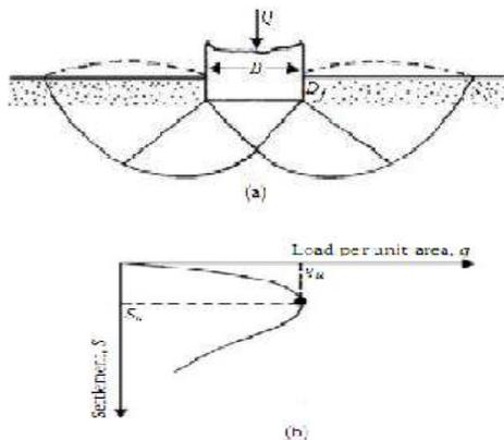
**Gambar 1** General Shear Failure
