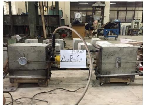
**Gambar 4.1** Pengujian *pull-out*
