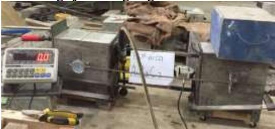
Gambar 4.2 Setting pengujian *pull-out*
