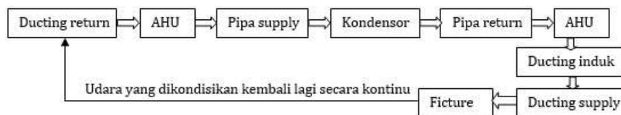
Gambar 8. Diagram Sistem Kerja *Split Duct*
