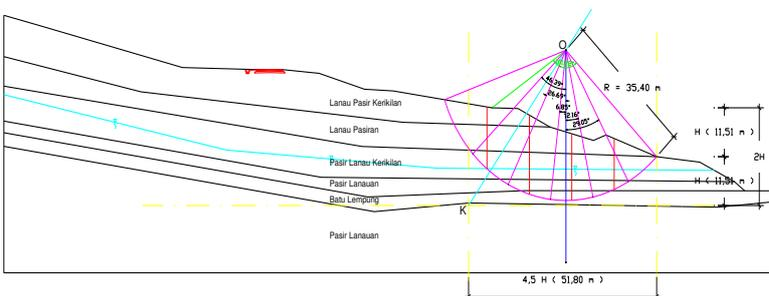
Gambar Cara Trial Error STA 0 + 275, R = 35,40 m
