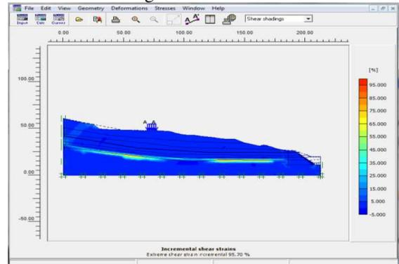
Gambar Incremental Shear Strains Tahap Cuting + Perkuatan Gabion
