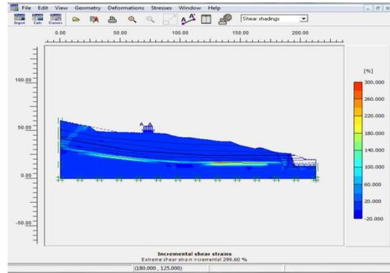
Gambar Incremental Shear Strains Tahap Cuting + Perkuatan DPT
