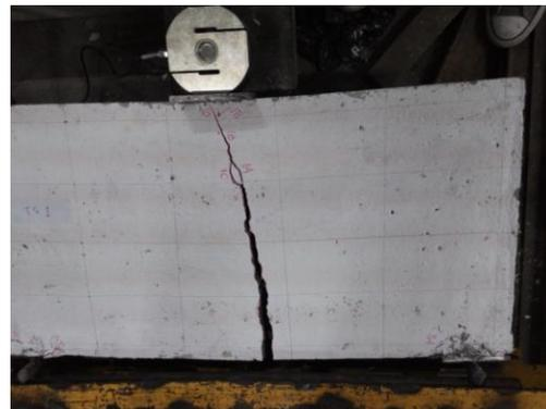
**Gambar 4.5 Model keruntuhan panel tanpa styrofoam**
