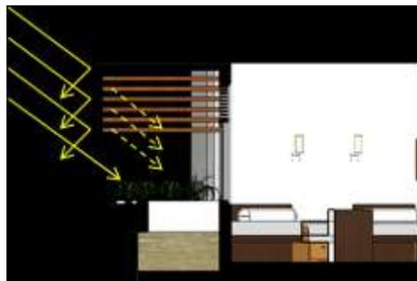
Gambar 4.48 Shading device terhadap sinar matahari
