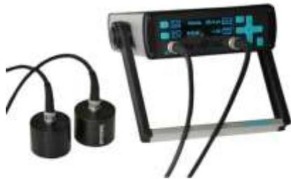
**Gambar 4.** *Ultrasonic Pulse Velocity(UPV)*
