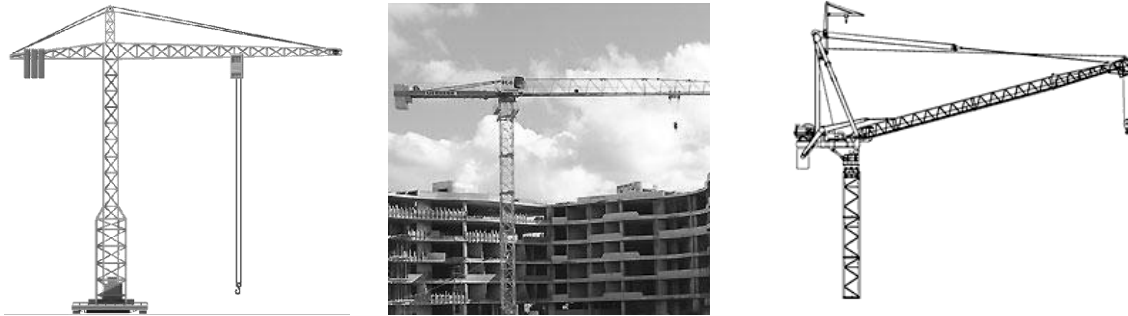
a. Hammer head crane
