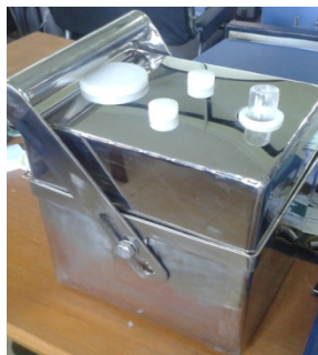
Gambar 6. Prototipe generator ^{99}\text{Mo}/^{99\text{m}}\text{Tc} berbasis kolom MBZ-Alumina
