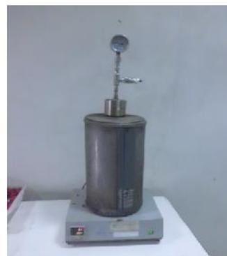
**Fig. 1.** The equipment scheme of the hydrothermal carbonization
