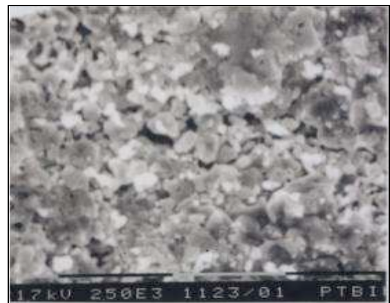
Gambar 4b. Struktur mikro konduktor padat (\text{CuI})_{0.7}(\text{AgI})_{0.3}
