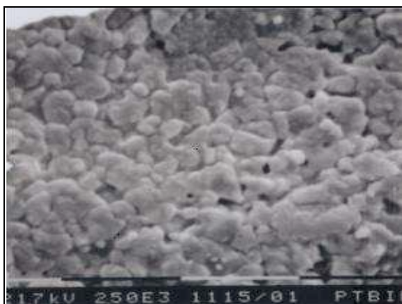
Gambar 4c. Struktur mikro konduktor padat (\text{CuI})_{0.9}(\text{AgI})_{0.1}
