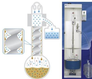
Gambar 1. *Spinning band distillation column*
