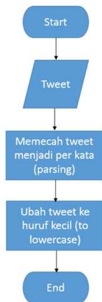
Gambar 3. Proses Pre-Processing Text
