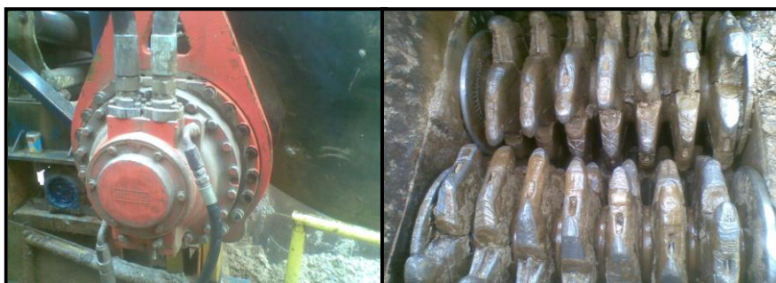
Gambar 2. Hydraulic Drive dan Twin Shaft Sizer
