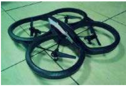
Figure 1. An AR.Drone quadcopter using indoor hull.
