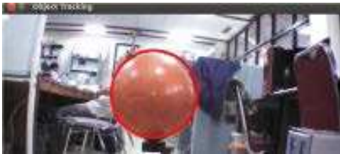
Figure 13. Object detected with distance of 0.5 meter.
