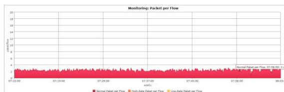
Fig 10. Packet per Flow Monitoring After Limiting Packets
