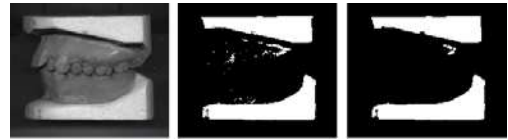
Figure 4. Example of resulted images (from left to right: grayscale, binary, and after morphology processes).
