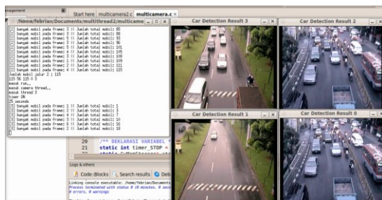
Figure 5. An example screenshot of a running program which is implemented vehicle object detection and tracking.
